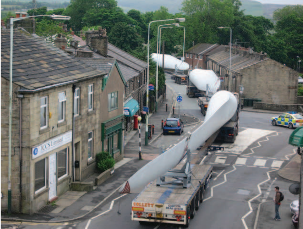
Notes: A convoy of wind turbine blades passing through the village of Edenfield, England. Photo Credit: Anderson (2007)
